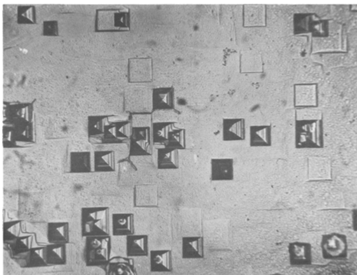
Figure 3 An etch pattern on the (001) cleavage face of SrFCl, \times 200 .
